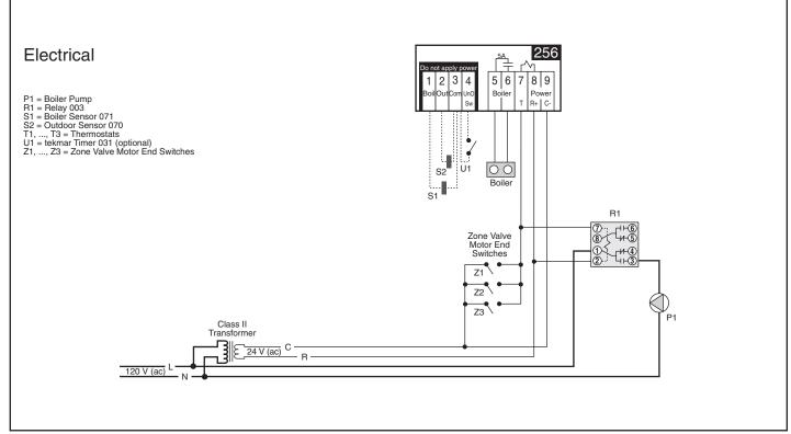
The Boiler Control 256 provides partial or full reset to three (or more) boiler zones. The boiler is operated at the temperature required in order to satisfy the load.
