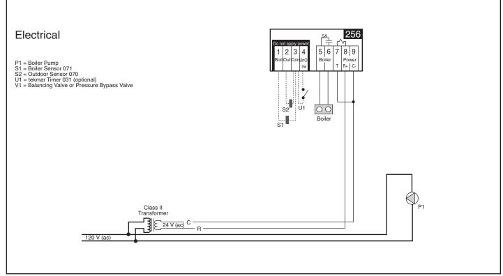
The Boiler Control 256 provides partial or full outdoor reset to four (or more) thermostatic radiator valve zones. Constant circulation to the system is provided by the boiler pump (P1). The boiler operates at the required temperature in order to satisfy the load.
