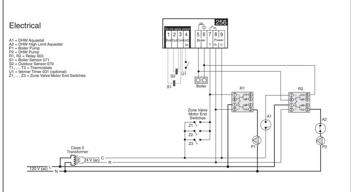
The Boiler Control 256 provides partial reset to three (or more) boiler zones. The supply of heat to an indirect Domestic Hot Water (DHW) tank is controlled through an external relay. The boiler operates at the required temperature in order to satisfy the loads.
