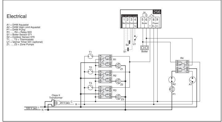
The Boiler Control 256 provides partial reset to three (or more) zones. The supply of heat to an indirect Domestic Hot Water (DHW) tank is controlled through an external relay. The boiler operates at the required temperature in order to satisfy the loads.
